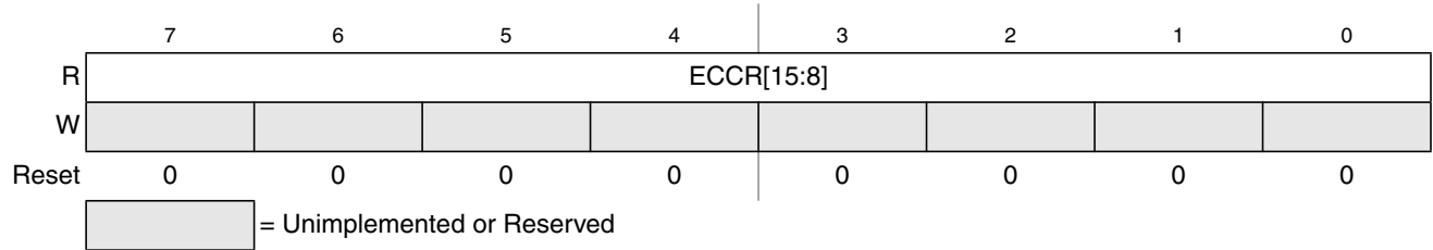
Figure 25-20. Flash ECC Error Results High Register (FECCRHI)
