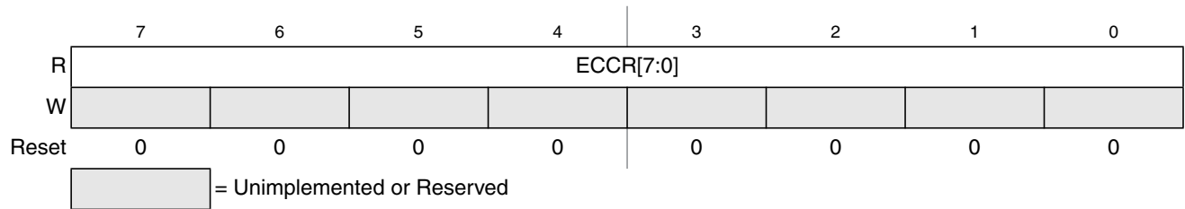
Figure 24-21. Flash ECC Error Results Low Register (FECCRLO)
