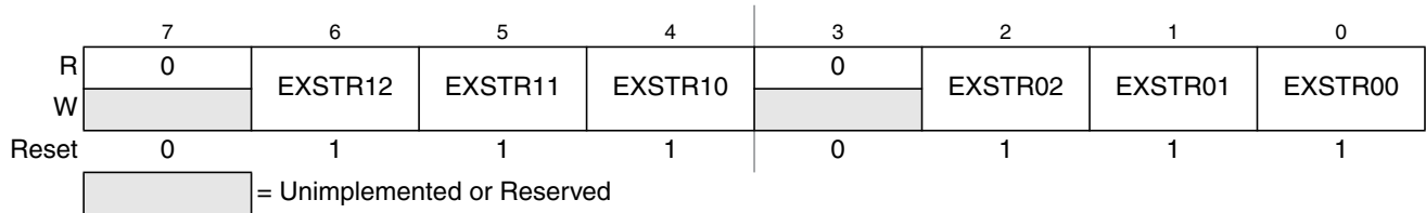
Figure 5-4. External Bus Interface Control Register 1 (EBICTL1)
