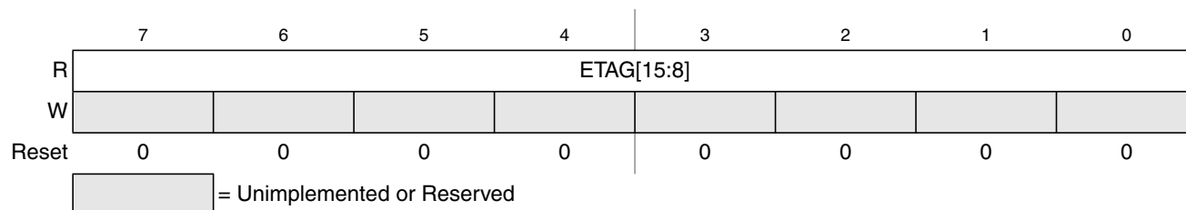
Figure 27-18. EEE Tag Counter High Register (ETAGHI)
