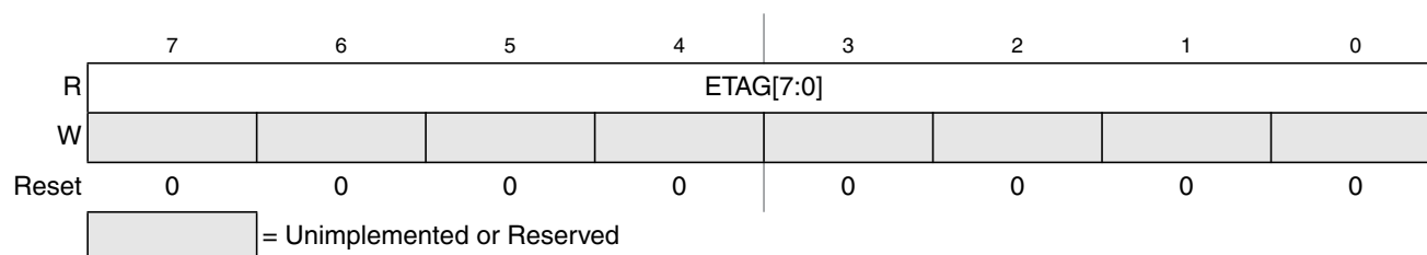
Figure 28-19. EEE Tag Counter Low Register (ETAGLO)
