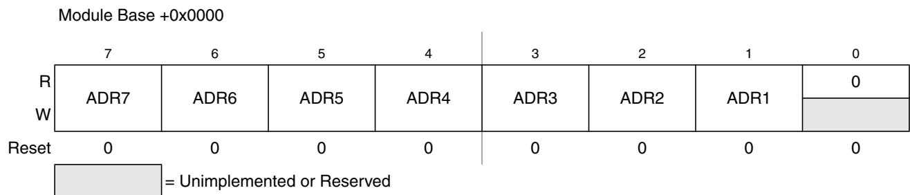
Figure 15-3. IIC Bus Address Register (IBAD)
