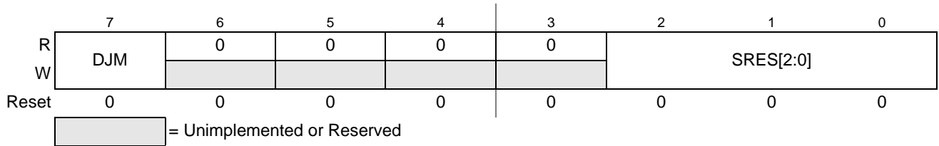
Figure 9-8. ADC Format Register (ADCFMT)
