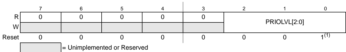
Figure 4-12. Interrupt Request Configuration Data Register 7 (INT_CFDATA7)
