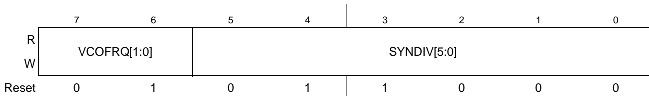
Figure 8-5. S12CPMU_UHV_V6 Synthesizer Register (CPMUSYNR)
