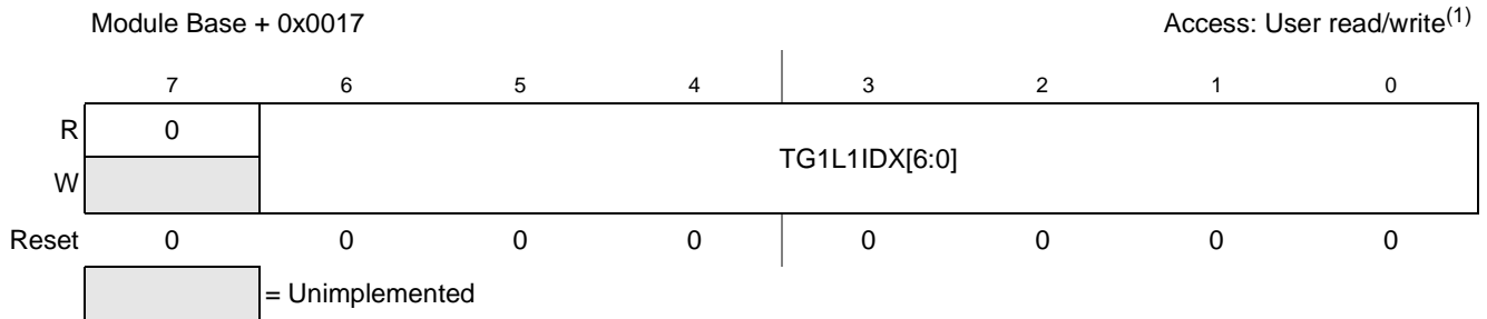
Figure 13-20. Trigger Generator 1 List 1 Index (TG1L1IDX)
