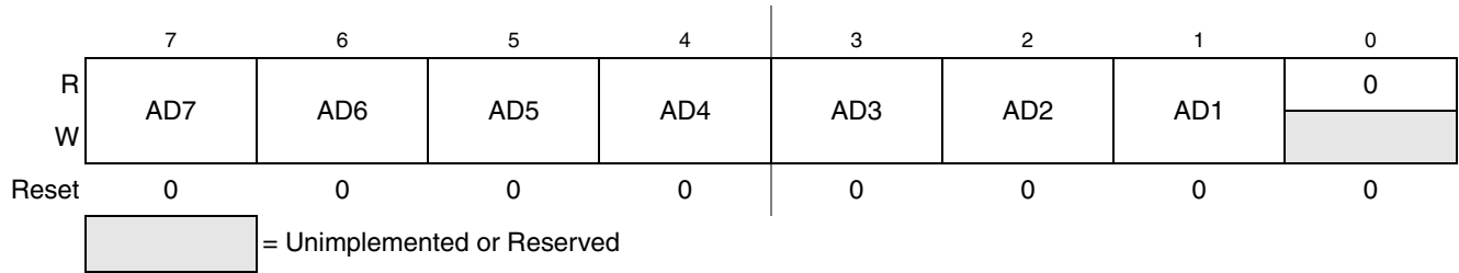
Figure 11-3. IIC Address Register (IICA)
