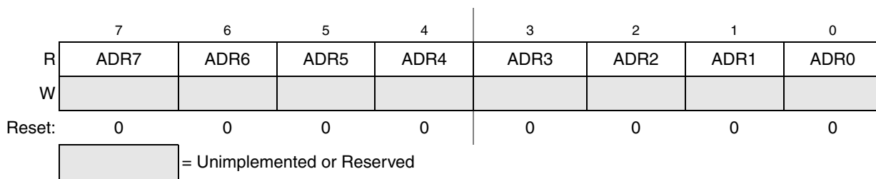
Figure 9-7. Data Result Low Register (ADCRL)
