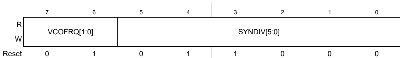
Figure 10-4. S12CPMU Synthesizer Register (CPMUSYNR)
