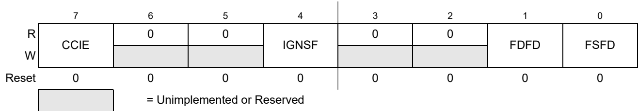
Figure 27-9. Flash Configuration Register (FCNFG)
