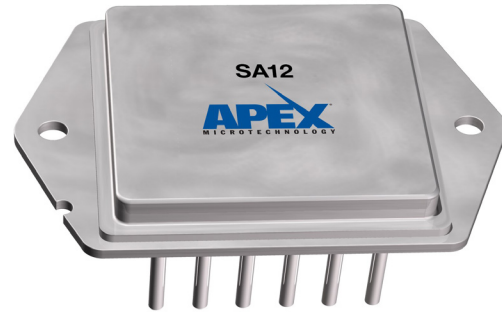
12-PIN POWER DIP PACKAGE STYLE CR
