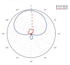
REALIZED GAIN PLOT Measured at 1575.42 MHz
