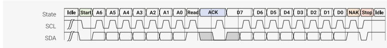
Figure 55. A 1-byte I2C read transfer. In the idle state, both lines float high. The initiator drives SDA low (a Start condition), followed by 7 address bits A6-A0, and a direction bit (Read/nWrite). The target drives SDA low to acknowledge the address (ACK). Data bytes follow. The target serialises data on SDA, clocked out by SCL. Every 9th clock, the initiator pulls SDA low to acknowledge the data, except on the last byte, where it leaves the line high (NAK). Releasing SDA whilst SCL is high is a Stop condition, returning the bus to idle.
