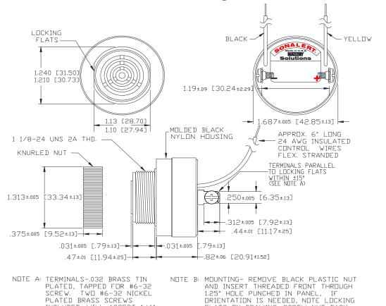
FLATS ON DRAWING, SCREW NUT BACK ON. DO NOT OVERTIGHTEN.
