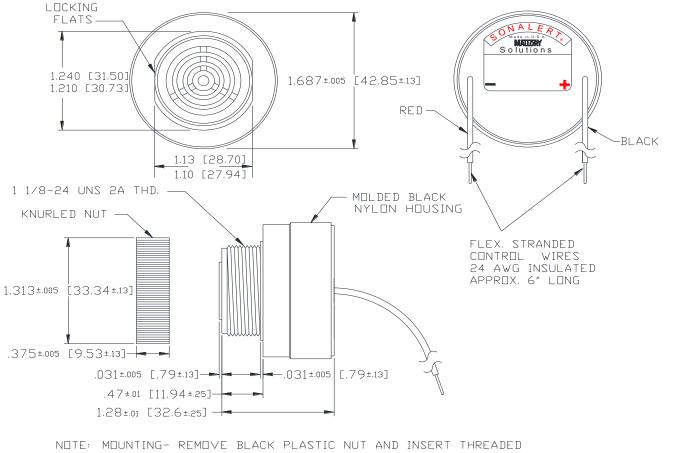
NOTE: MOUNTING- REMOVE BLACK PLASTIC NUT AND INSERT THREADED FRONT THROUGH 1.25" HOLE PUNCHED IN PANEL, IF ORIENTATION IS NEEDED, NOTE LOCKING FLATS ON DRAWING. SCREW NUT BACK ON. DO NOT OVERTIGHTEN.
