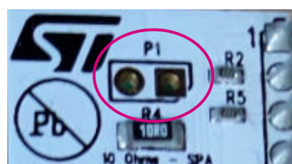
Figure 5. P1 header location
