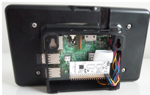
Figure 4. STPM4RasPI embedded in the Raspberry Pi box with touch screen
