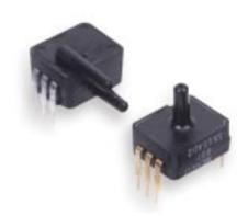
The SDX series sensors provide a very cost effective solution for pressure applications that require small size plus performance. These calibrated and temperature compensated sensors give an accurate and stable output over a 0°C to 50°C temperature range. This series is intended for use with non-corrosive, non-ionic working fluids such as air, dry gases and the like.
