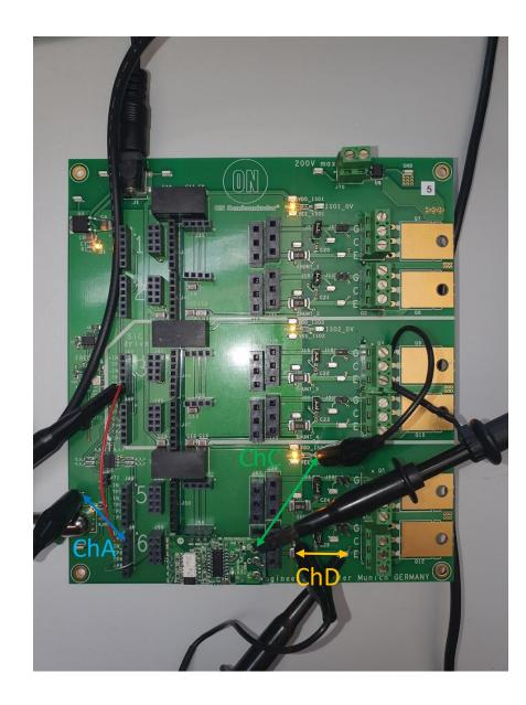
ChA: Measure voltage across J58.1 and GND on test point close to BNC connector
