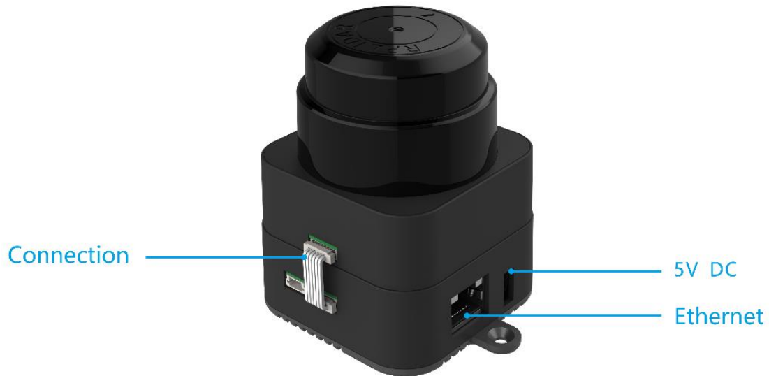
Figure 2-5 SLAMTEC Mapper Professional Kit Interface Definition Diagram
