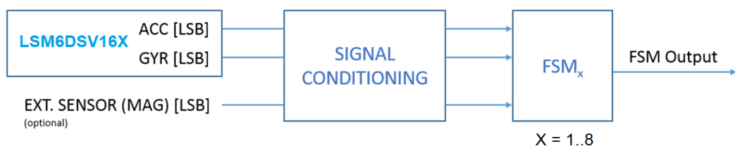
Figure 3. State machine in the LSM6DSV16X
