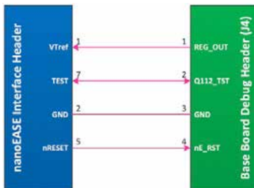
Figure 38: nanoEASE - Base Board Connection Diagram
