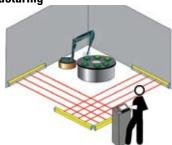
**Situation**: Protect operator from being hit or crushed by a robotic arm's movement.
