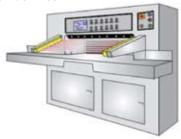
**Situation**: These machines typically cut paper to a specific size for newspapers or special applications and the operator needs to be protected against injury from the cutter blades.
