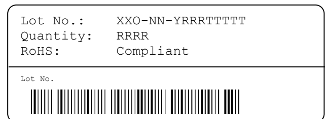
Figure 22: First label on reel: XX = Sensor Type (20 for SHT20), O = Output mode (D = Digital, P = PWM, S = SDM), NN = product revision no., Y = last digit of year, RRR = number of sensors on reel divided by 10 (200 for 2000 units), TTTT = Traceability Code.
