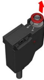
Figure 14. Remove the plastic washer
