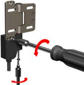
Figure 11. Remove the screws
