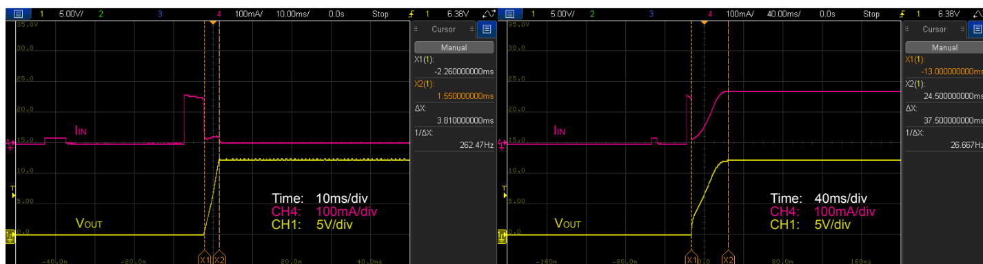
Figure 6.7. Si3406-Buck Non-Isolated EVB, 12 V, Class 2 Output Voltage Soft-Start at Low-Load (Left) and Heavy-Load (Right) Conditions
