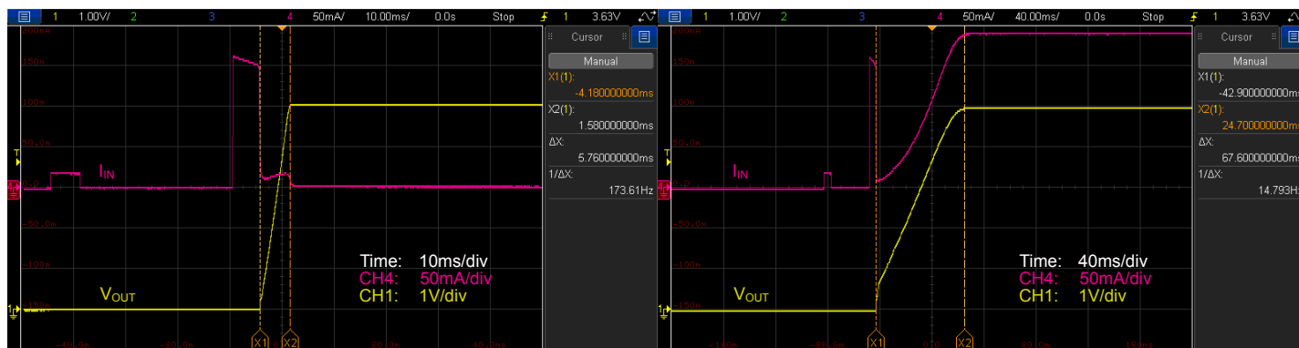
Figure 5.7. Si3406-Buck Non-Isolated EVB, 5 V, Class 2 Output Voltage Soft-Start at Low Load (Left) and Heavy Load (Right) Conditions
