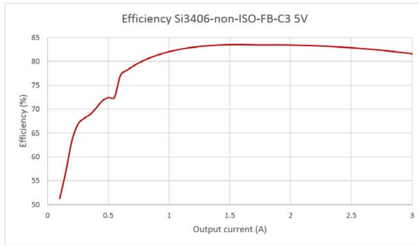
Figure 3.1. Si3406-Non-Isolated Flyback Class 3 EVB Overall Efficiency: 50 V Input, 5 V Output, Class 3 PD
