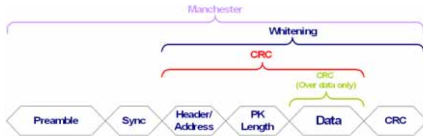
Figure 23. Operation of Data Whitening, Manchester Encoding, and CRC
