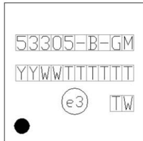
Figure 8.6. Si53305 Top Marking
