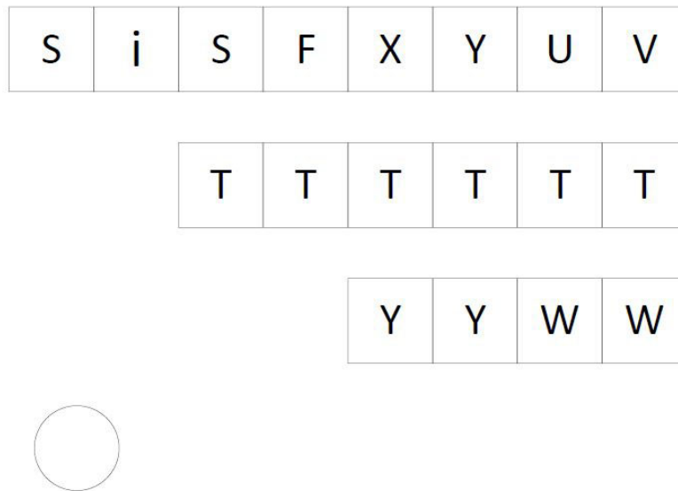
Figure 34. SSO-8 Top Marking
