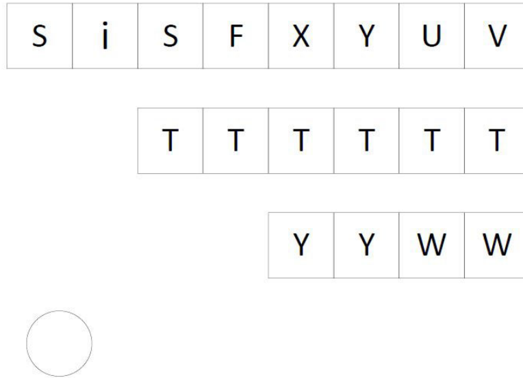
Figure 34. SSO-8 Top Marking
