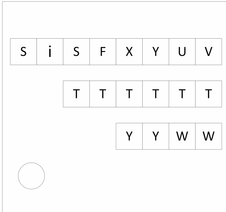
Figure 16. SSO-8 Top Marking
