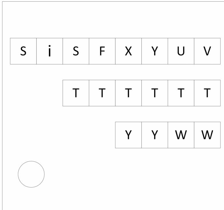
Figure 16. SSO-8 Top Marking
