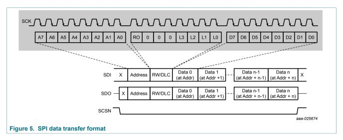
The SJA1124 monitors the number of data bits transmitted. If the number of bits is not between 24 and 144, is not a factor of 8, or the number of bytes does not match the DLC in the SPI conrol byte, the write access is ignored and an SPI error interrupt (SPIEI) is triggered (see <u>Table 22</u>).
