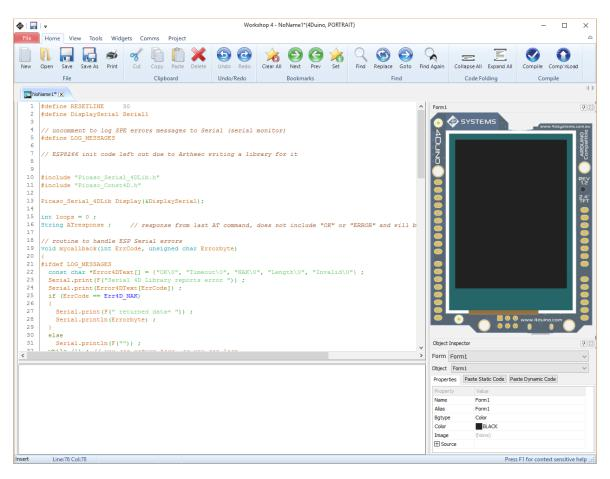
4D Arduino - Basic Graphics is designed primarily for use when no uSD card will be used with the display. Graphics primitives can be dragged and dropped onto the screen and the place in your code where the primitive is to be used can be located and the code pasted into the editor.
