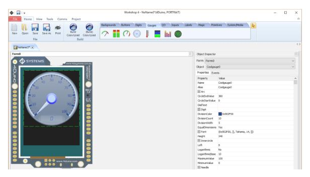
Each object has parameters that can be set, such as colour, range, text, etc. It is then just a case of selecting the event the object is to be associated with -- such as sending the value to the Atmel or directly interfacing to another object, it is that simple. In seconds you can transform a blank display into a fully animated GUI with moving sliders, animated press and release buttons, and much more.
