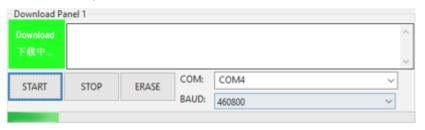
• Then the application will load and the ESP8266 is wiped blank. It will complete when the progress bar goes to the very right-hand side.
