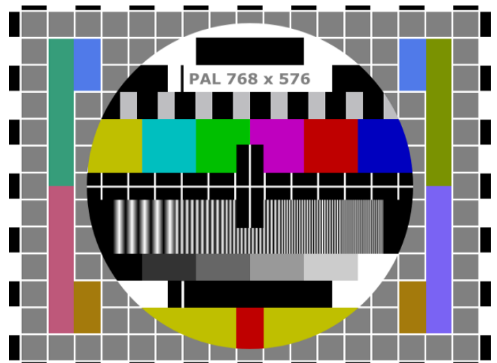
Figure 5: Output frame from the hardware simulation example (Scale-down of 768x576 to 640x480)
