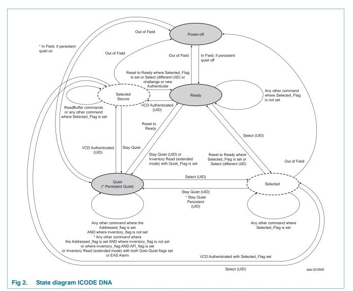
**Remark:** It is possible to set the ICODE DNA IC into the Quiet and Persistent Quiet mode at the same time. In this case the behavior is the same as for the Quiet state only until the IC enters the Power-off state. The IC enters to the Persistent Quiet mode at the next power-on if the persistent time has not been exceeded.
