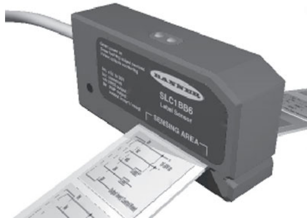
Figure 2. Allowing the web to glide over the bottom fork with slight tension lessens the effects of web flutter.
