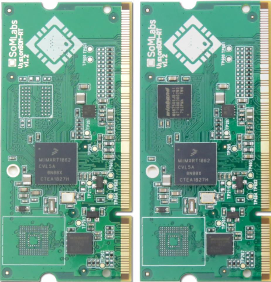
The VisionSOM-RT family is a SODIMM-sized SoM based on the NXP i.MX RT application processor which features an advanced implementation of a single ARM Cortex-M7 core (at speeds up to 600MHz).
