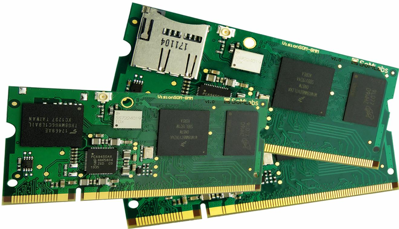
The VisionSOM-8Mmini family is a SODIMM-sized SoM based on the NXP quad core i.MX8M mini application processor which features an advanced implementation of a single or four ARM Cortex-A53 cores (at speed up to 1.8GHz) and ARM Cortex-M4 core (at speed up to 400MHz) as well as a 2D (HD1080p60) and 3D Graphics Processing Unit (GPU) Open GL 2.0 ES compatible and Video Processing Unit (VPU) with D1080p60 H.264 and HD1080p60 H.265 capabilities.
