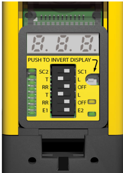
Figure 26. EZ-SCREEN Configuration DIP Switches (Receiver)
