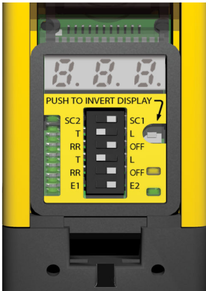
Figure 26. EZ-SCREEN Configuration DIP Switches (Receiver)
