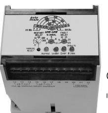
The ATC-Diversified Electronics SLU-600-ASTDS Universal Phase Monitor protects 3-phase motors up to 700VAC. The RAPID CYCLING feature prevents motors cycling due to load-induced line fault conditions. Powered by 120VAC, this reliable motor protection relay is unaffected by transients and disturbances from the monitored power source. The SLU-600 Series is UL Listed under UL File Number E55826.
