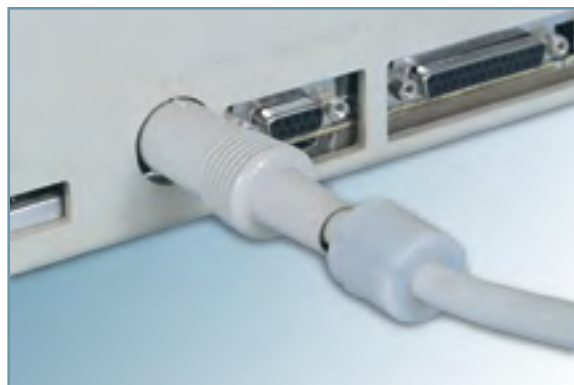
I/O cable with RFI suppressor.
