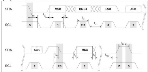
$<sup>^{\</sup>star\star}$ ) For I²C bus capacitance load >100pF maximum possible clock frequency is 100kHz
