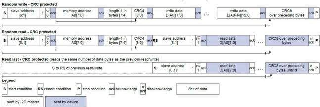
The memory address field sets the byte address of the first memory location to be read from or written to. Only 16-bit-word aligned reads/writes are supported, i.e. the LSB of memory address has to be zero always. The read/write data is transferred MSB first, low byte before high byte.
