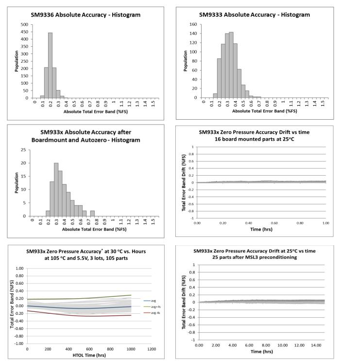
Zero pressure total error band tested at 30 °C and 3.3V. Measured after HTOL (at 105 °C and 5.5V) at 168, 500 and 1000 hrs. Not tested in production
