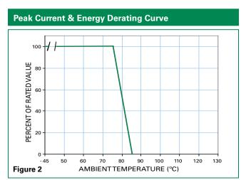
For applications exceeding 75°C ambient temperature, the peak surge current and energy ratings must be reduced as shown.
