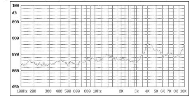
Typical Frequency Response (3Vp-p sine-sweep with microphone spaced at 10cm)
