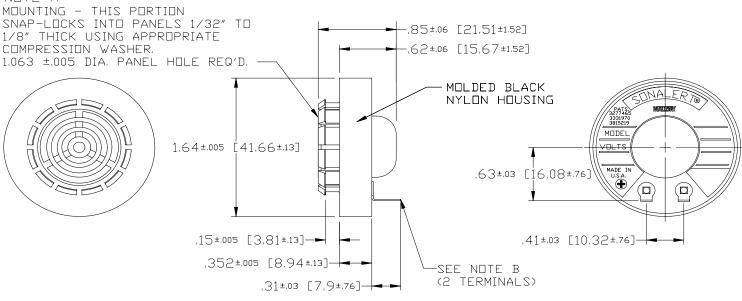
NOTE B: TERMINALS - .016 BRASS, HOT TIN FINISH WITH .076 WIRE HOLE, TERMINAL WILL ACCEPT STANDARD 1/8" QUICK CONNECT
