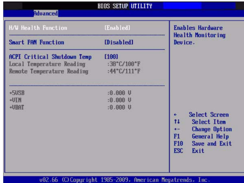
Figure 3.15 Hardware Health Configuration
