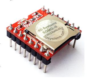
Audio files can be easily loaded to the micro-SD card or USB Flash drive using a PC/Laptop, and inserted into the SOMO-II for playback. No external software is required.
