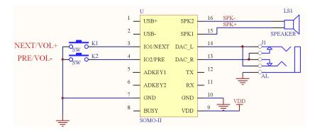
This is an example schematic showing the simplest connections to the SOMO-II for KEY MODE. Only 2 buttons are required. NEXT/VOL+ will start playing a track if currently stopped, and will raise the volume if the button is held down for > 1.2 seconds. PRE/VOL- will start playing a track if currently stopped also, and will lower the volume if the button is held down for > 1.2 seconds. See the table under the KEY MODE for more information.
