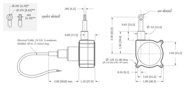
DIMENSIONS ARE IN INCHES [MM] tolerances are 0.04 IN. [1,0 MM] unless otherwise noted.
