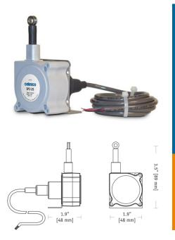
The SP2 String Pot from Celesco is a compact, economical and water resistant device that utilizes a flexible cable, a spring-loaded spool and a potentiometer to detect and measure linear position.
