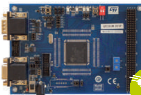
Discovery Kit for the M Line with SPC56M64L7. order code: SPC56M-DISP
