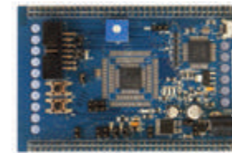
SPC56D-Discovery with SPC56D40L1 order code: SPC56D-DIS
